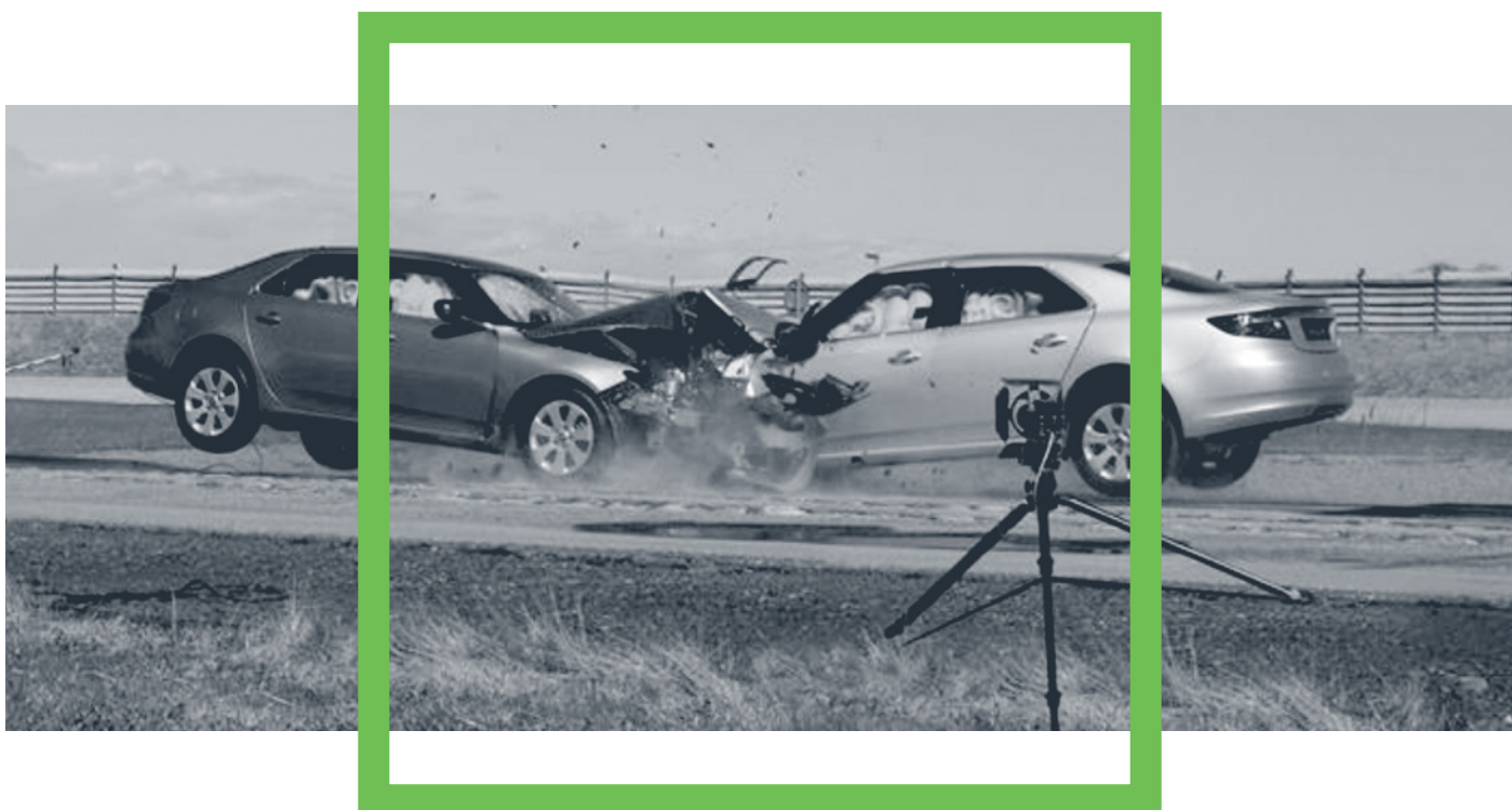
Saab 9-5 (Epsilon II) impacted corner to corner at 60 km/h on a test track, to prove the occupant protection systems really do work.
